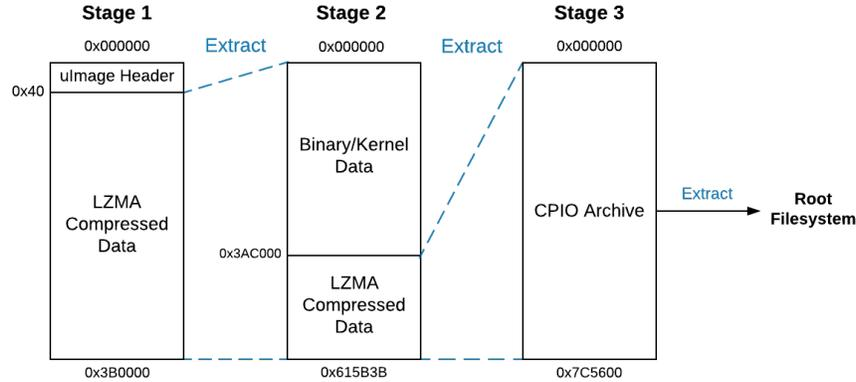
**Fig. 1.** Extracting the DCS-932L’s Root Filesystem from the Kernel Partition
