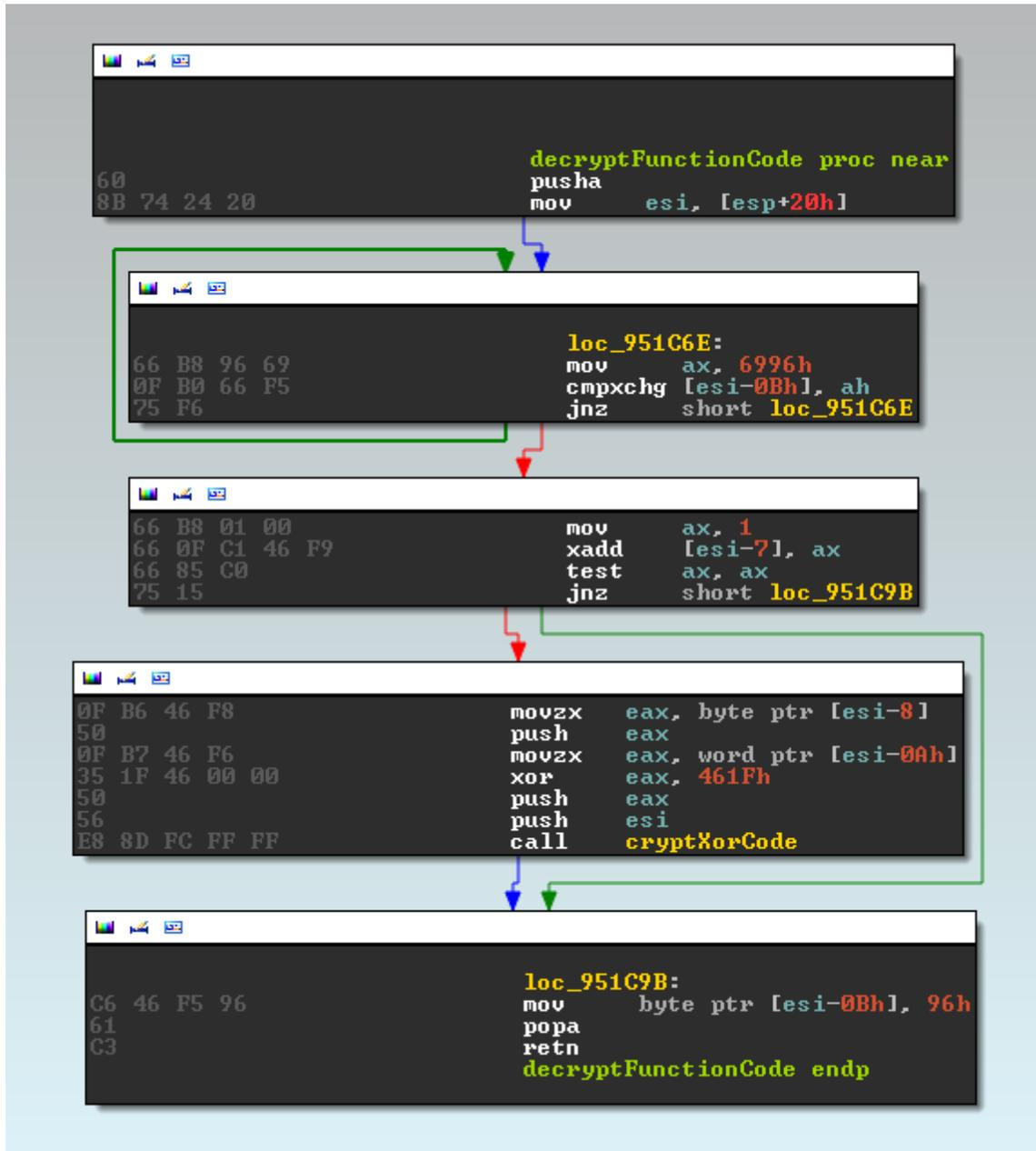
Fobber's on-demand decryption code for functions, revealing the parameter offsets necessary for decryption.
