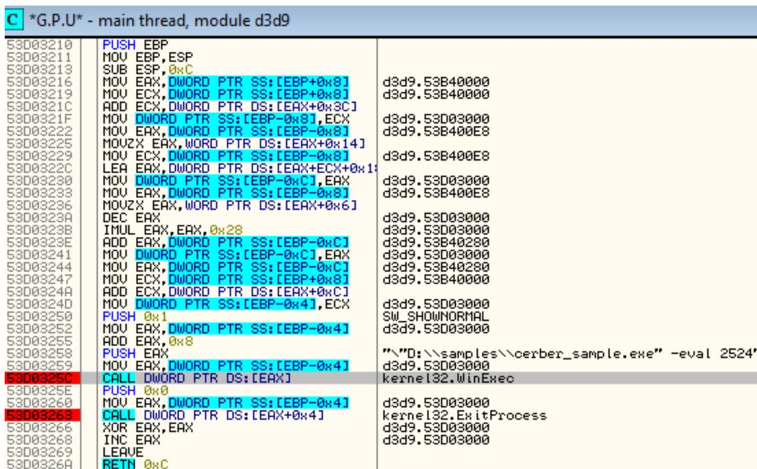
Successful UAC bypass is signaled by setting a property named “cerber\_uac\_status” in a found window of the class “Shell\_TrayWnd”. The initial Cerber sample waits for this status to change. If the timeout passed and it didn’t changed it makes a new attempt of UAC bypass – using a different pair (EXE+DLL). Otherwise it cleans up the environment and terminates. Infection proceeds from inside of the elevated sample.
