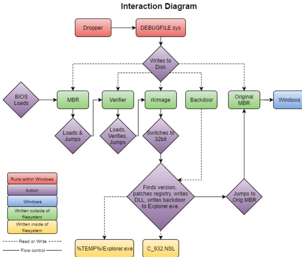
Figure 9: Diagram showing the out-of-OS boot process.
