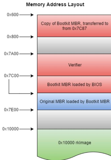
Figure 7: Address layout of memory loaded before rklmage
