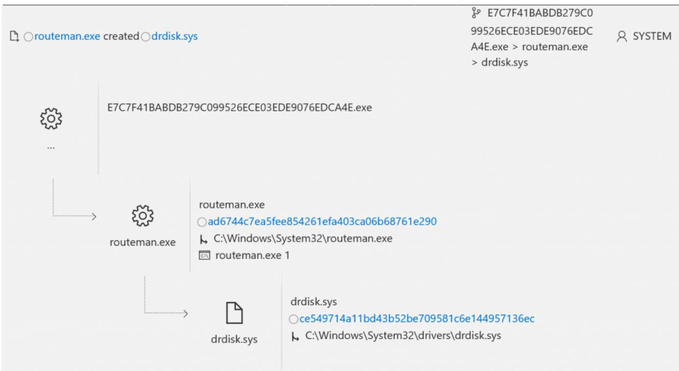
Figure 3. Windows Defender ATP event tree: Depriz Trojan dropping the wiper component (named “routeman” in this instance), which in turn drops the RawDisk driver “drdisk”
