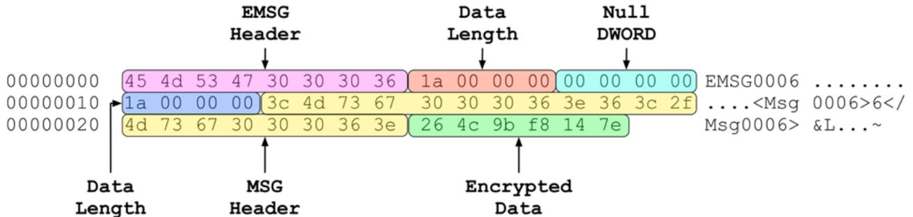
Figure 2 MoonWind network communication packet format
