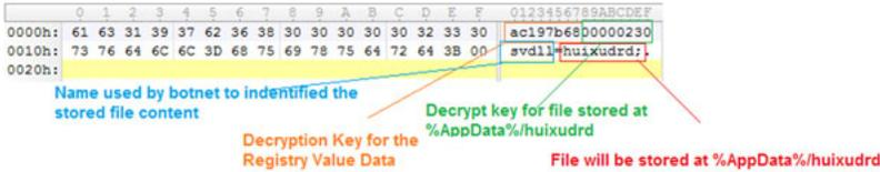
Figure 5. Registry data reveals information after decryption (XOR with DWORD key).
