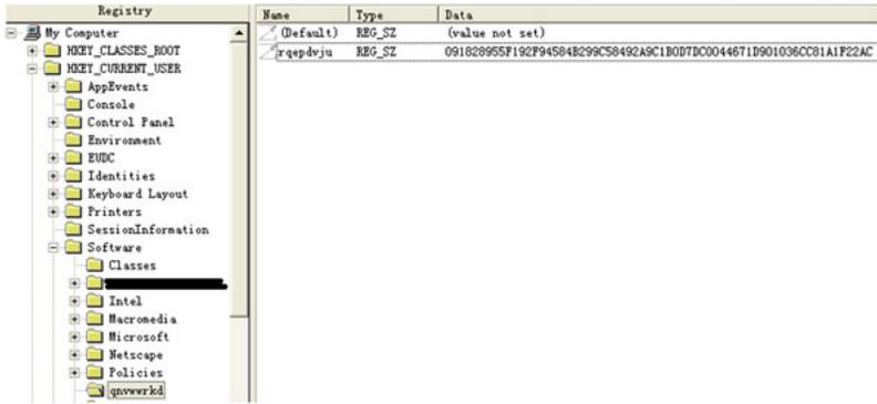
Figure 4. Registry of a host infected by Sasis.
