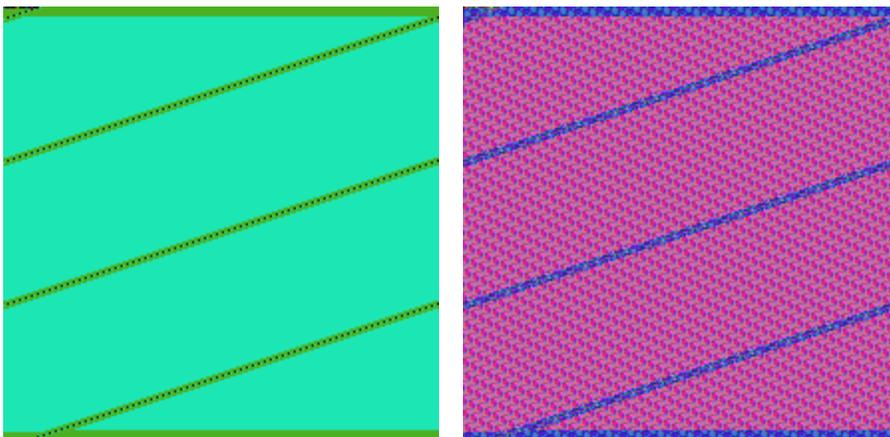
We can see the patterns of the original file reflected in it's encrypted content. Such an effect depicts, that file could have been encrypted by some block cipher – but as well it can be a custom, XOR-based algorithm.
