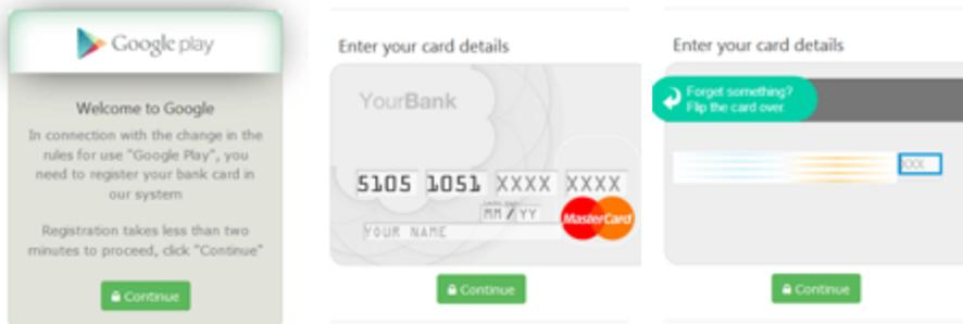
When an SMS message arrives, the Trojan turns off all sounds and vibrations, sends the message content to the cybercriminals, and attempts to delete the original messages from the list of incoming SMS. As a result, a user could miss not only bank notifications about the unplanned transactions but also other incoming messages.
