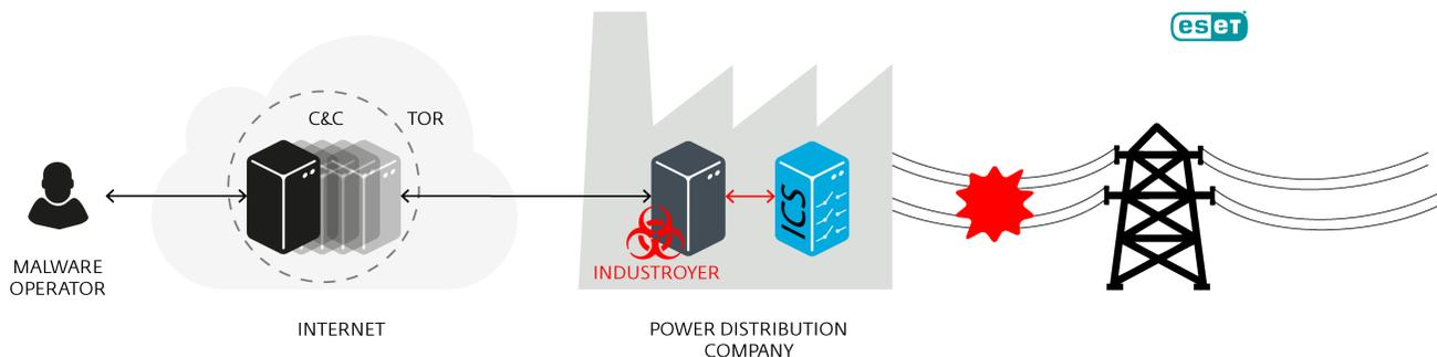
Industroyer is a particularly dangerous threat, since it is capable of controlling electricity substation switches and circuit breakers directly. To do so, it uses industrial communication protocols used worldwide in power supply infrastructure, transportation control systems, and other critical infrastructure systems (such as water and gas).
