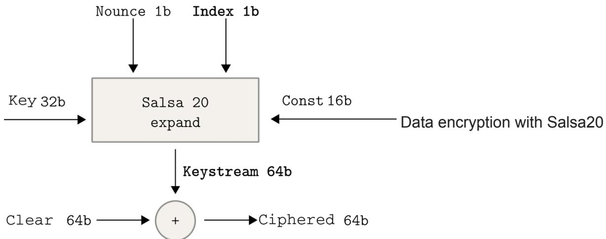
We can verify this using Miasm, by looking at the data before and after encryption, and by showing their XOR difference.
